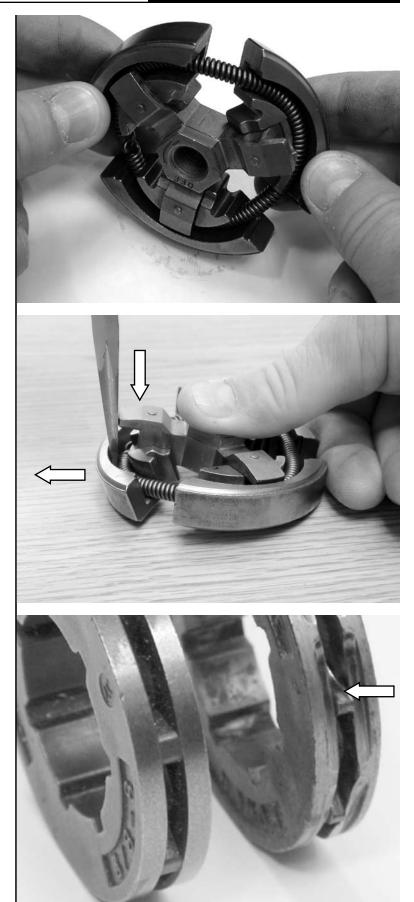
7.8 Finish installation of clutch shoe as shown.
